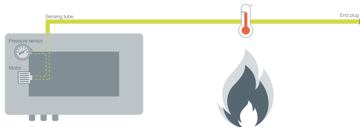
Operating principle of ADW 535
