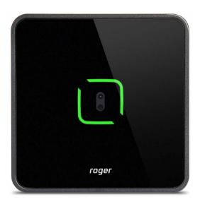
CEB12 is a contactless button which, after recognizing that the hand is approaching the front panel, temporarily switches on its electrical output. CEB12 can be connected to the access controller controlling the door or directly, without the access controller, to the electric door strike.
