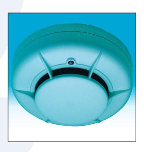
The HRZ-1003 detector has an integral LED, which illuminates to provide a local alarm signal. This latches on, and remains illuminated until the detector is reset by a momentary power interruption. An optional remote LED annunciator may be used to repeat any alarm signal.
