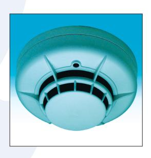
The HRZ-1005T detector also has an integral LED, which illuminates to provide a local alarm signal. This latches on, and remains illuminated until the detector is reset by a momentary power interruption. An optional remote LED annunciator may be used to repeat any alarm signal.
