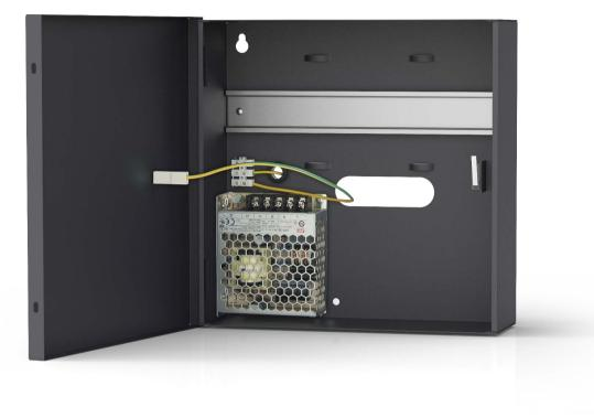
The ME-14-24V enclosure is dedicated to RACS 5 modules and devices which require installation on DIN rail and 7 Ah battery. The enclosure is equipped with a single DIN rail, DC power supply and tamper contact. Access to the internal space of the enclosure is protected by a door fixed by screws. The ME-14-24V is made from a metal sheet painted with an anthracite grey powder coating (RAL7016).
