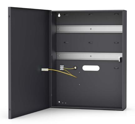
The ME-17 enclosure is dedicated to RACS 5 modules and devices which require installation on DIN rail and 17 Ah battery. The enclosure is equipped with 2 DIN rails and tamper contact. Access to the internal space of the enclosure is protected by a door fixed by screws. ME-17 is made from a metal sheet painted with an anthracite grey powder coating (RAL7016).
