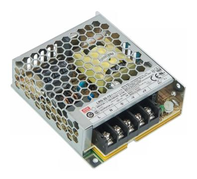
PS2D is LRS-35-12 (Mean Well) power supply unit with rated output voltage increased from 12.0 V to 13.8 V by means of originally available output potentiometer. PS2D is dedicated to installation in RACS 5 system, particularly to supply MCX2D and MCX4D expanders and PSD4D power distributors but it can also be used for other applications if its nominal conditions of use are
