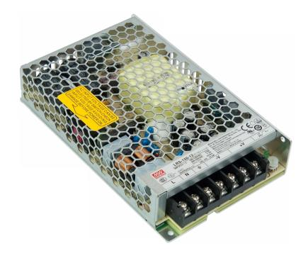
PS8D is LRS-150-12 (Mean Well) power supply unit with rated output voltage increased from 12.0 V to 13.8 V by means of original output potentiometer. PS8D is dedicated to installation in RACS 5 system, particularly to supply MCX2D and MCX4D expanders and PSD4D power distributors but it can also be used for other applications if its nominal conditions of use are satisfied. The PSU is
