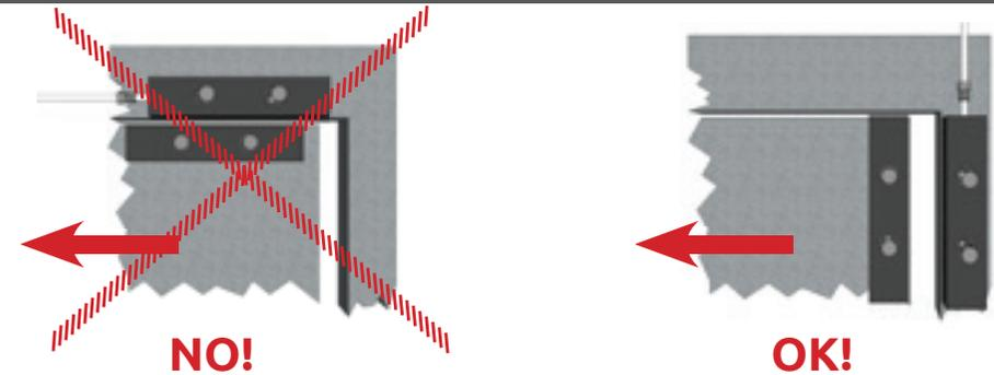
\* Installation on sliding doors requires mounting sensor and magnet as shown in the picture above on the right. In practice, care must be taken so that when the door is opening and closing the magnet does not slide from/to the sensor.
