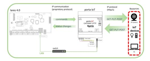
**porta IoT** is connected to the control panel via LAN through ethernet port. It can be powered by PoE or by external power supply (12/24Vdc). It is supplied with a plastic box that occupies 4 DIM modules.
